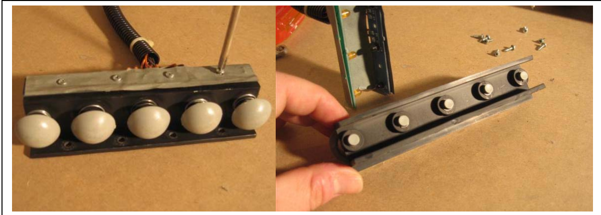
Figure 29 Correctly Assembled Mushroom Plunger in the housing
