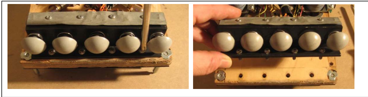
Figure 21 Remove the Five Button Opto Assembly from the MPF
