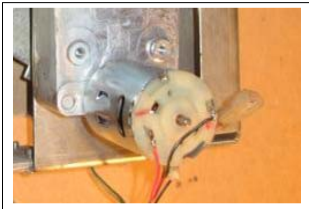
Figure 20 Wiring the motor
