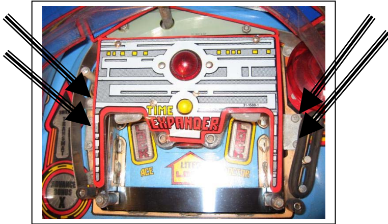
Figure 8 Remove MPF Retaining Screws
