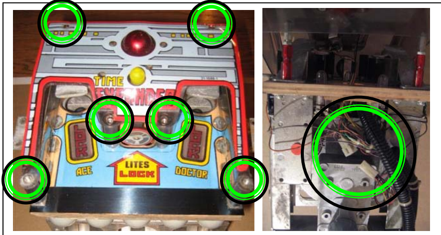
Figure 11 Removing the MPF Cover Assembly [Screw locations and connector]
